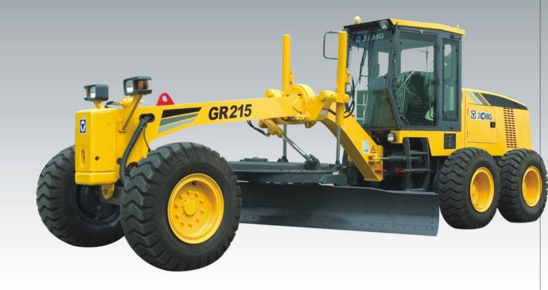
Weight 17000kg 153kw(205HP) Rated Power 4270mm Blade Width
