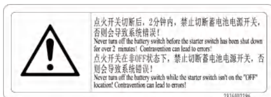
29. Main power switch warning sign
